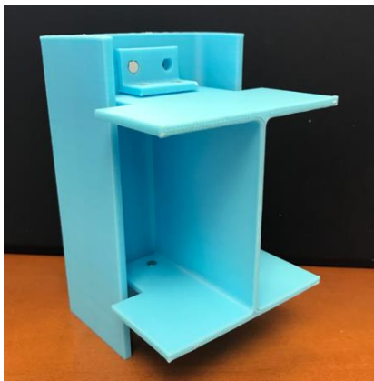
(e) Connection 5 – Unstiffened Seated Connection
