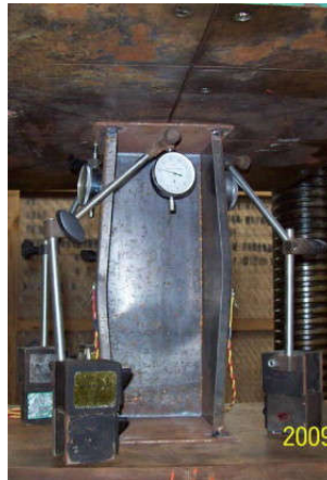
Stub column test where actual residual stresses impact stress-strain curve
