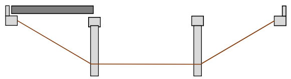
Simple 3-Span Precast Girder Bridge
