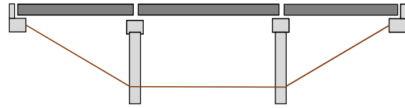
Simple 3-Span Precast Girder Bridge
