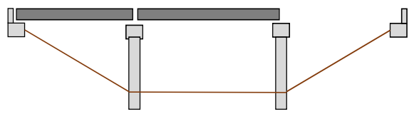
Simple 3-Span Precast Girder Bridge
