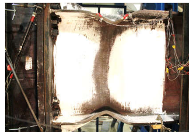
End Plate Moment Connection Subjected to Large Cyclic Deformations
