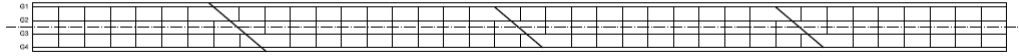
Bridge 13 ( L_s = 185 ft, 253 ft, 253 ft, 186 ft; w_g = 36 ft; \theta = 0^\circ, 50.1^\circ, 50.1^\circ, 50.1^\circ, 0^\circ ; I_s = 0.23 ; O_{min}/b_f = 2.40 )
