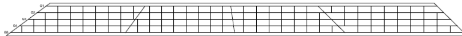
Bridge 15 ( L_s = 188 ft, 156 ft, 159 ft, 226 ft; w_g = 49.2 ft; \theta = 53.4^\circ, 36.2^\circ, 8^\circ, 45.3^\circ, 45.3^\circ ; I_s = 0.32 ; O_{min}/b_f = 1.45 )
