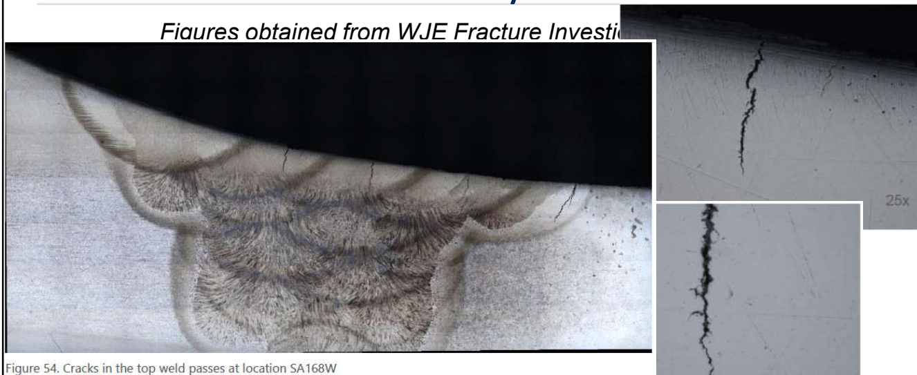
Figure 54. Cracks in the top weld passes at location SA168W
