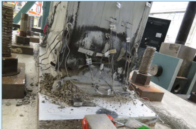
Fracture Failure During 6 \Delta y Cycles – Point E
