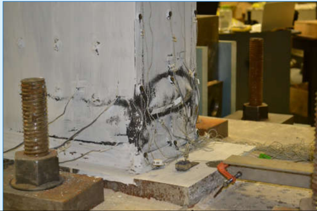
Photographs of Local Buckling During 3 \Delta y Cycles – Point C
