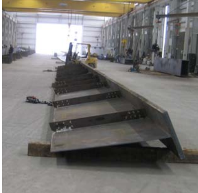
Flanges and Connection Plates Welded to Web
