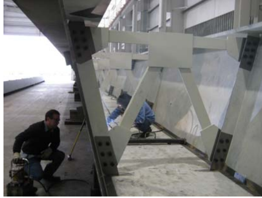
Cross Frames Used to Control Box Geometry
