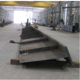
Flanges and Connection Plates Welded to Web
