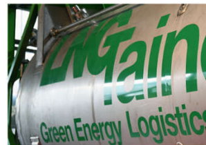
Liquefied natural gas (LNG) tanks made from austenitic stainless steel
