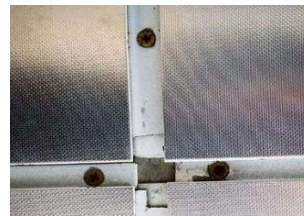
Rapidly corroding galvanized steel bolts – no impact on stainless steel!
