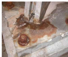
Rapidly corroding galvanized steel bolts – no impact on stainless steel!
