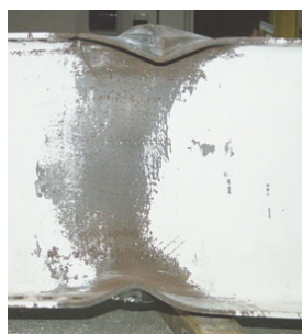
Local Flange Buckling (LFB)
