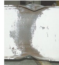
Local Flange Buckling (LFB)
