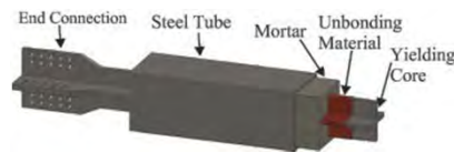
Buckling restrained brace, sciencedirect.com
