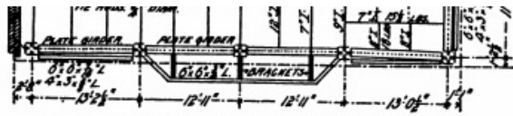
FIG. 19.—Typical Framing Plan of the Reliance Building.
