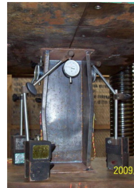
Stub column test where actual residual stresses impact stress-strain curve
