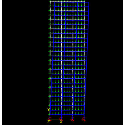
Deflected Shape: 2 10 -Order Elastic, Incr # 20, Applied Load Ratio = 1
