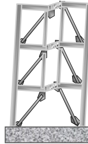
Braced frame with constrained story drifts
