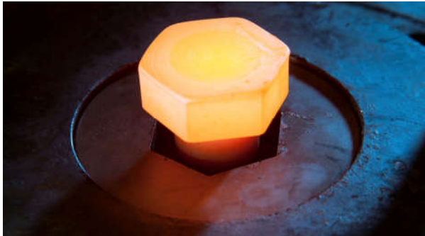
Bolt Hot Forging
