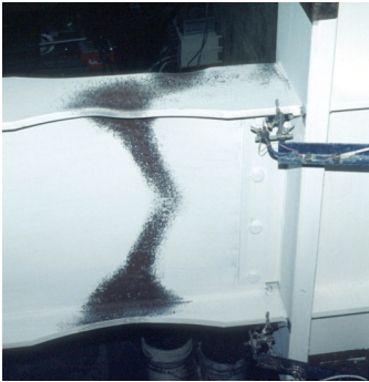
Yielding in moment frame beam (plastic hinge)
